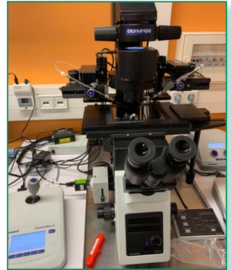
Micromanipulation work station
